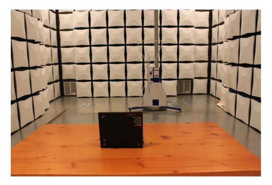
1.2.Photos of Radiated Emission Test (30-1000MHz)
