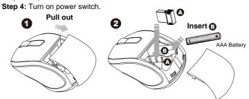
\*\*Warning: \*Please insert the battery with the correct position according to the instruction labeled on the mouse.
