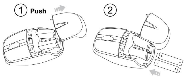
For Extra usage hours, use two AA batteries instead of two AAA Batteries.
