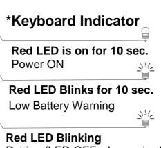
Pairing (LED OFF when paired or failed after 10 sec.)
