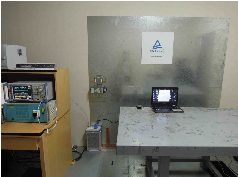
Photograph 5: Set-up for for Mains Conducted testing Front
