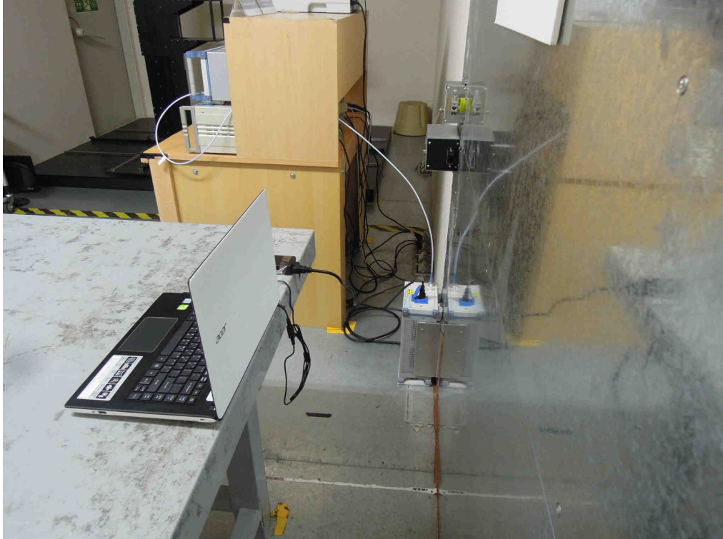
Photograph 4: Set-up for for Mains Conducted testing Back
