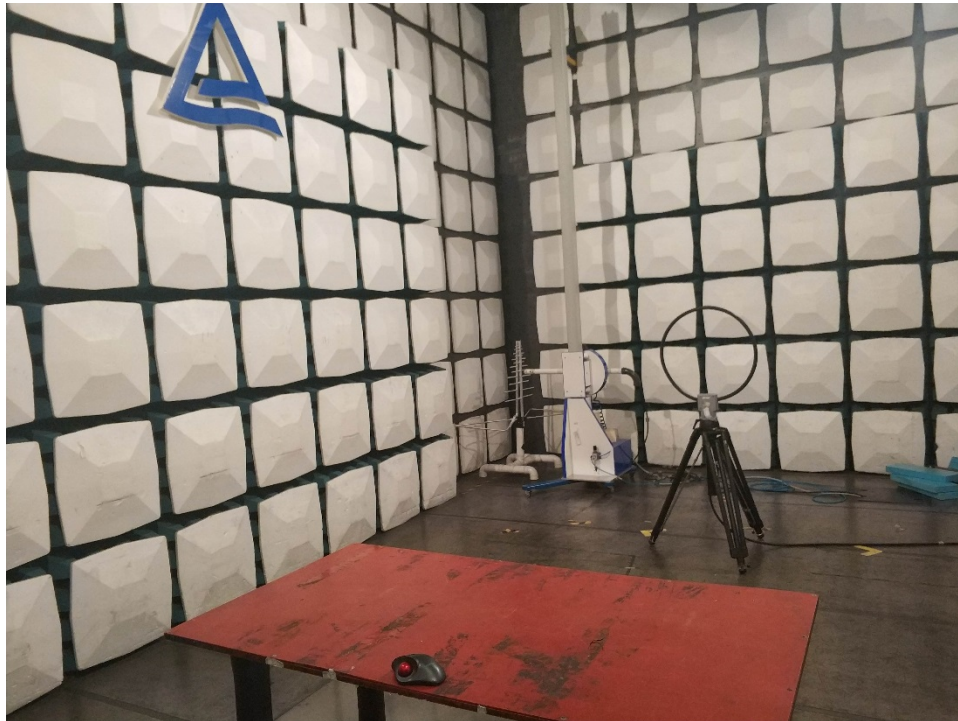
Photograph 1: Set-up for Radiated Spurious Emission, 9kHz - 30MHz
