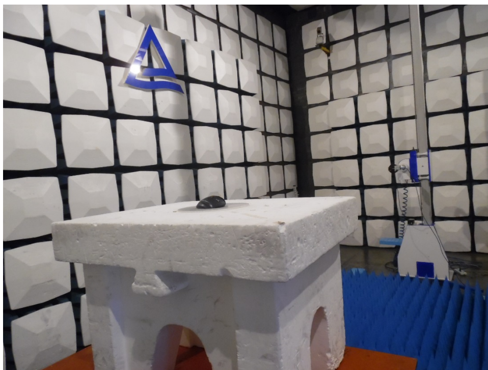
Photograph 4: Set-up for Radiated Spurious Emission, 18GHz - 26.5GHz
