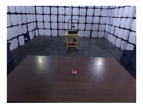
Radiation Emission Test Setup (30MHz to 1GHz)
