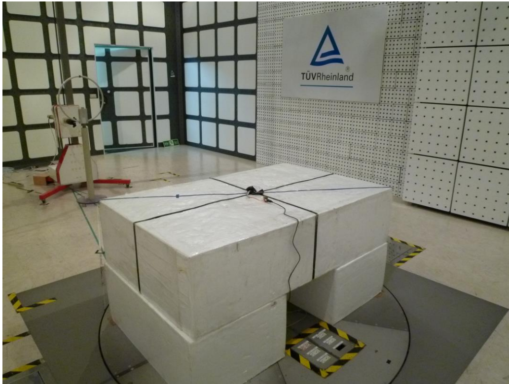
Photograph 4: Set-up for Spurious Emissions (Back View 3)
