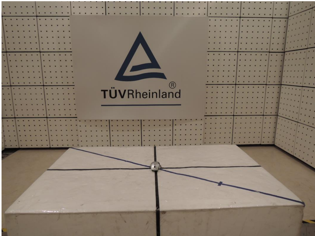
Photograph 1: Set-up for Spurious Emissions (Front View)
