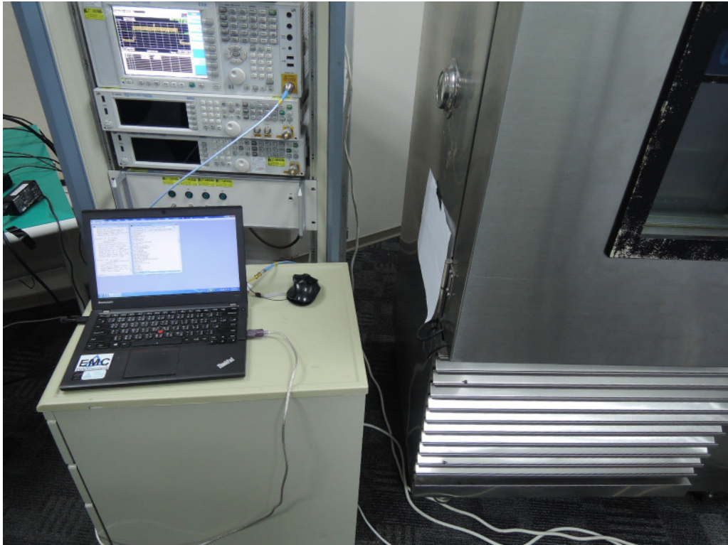
Photograph 4: Set-up for Conducted testing
