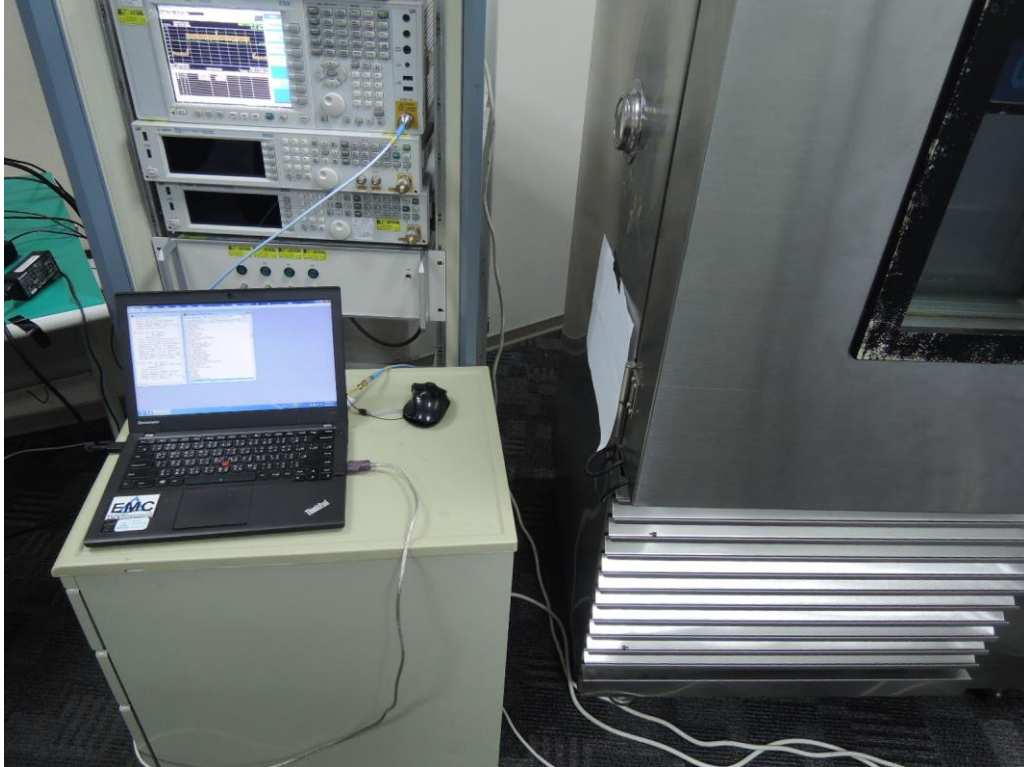
Photograph 4: Set-up for Conducted testing
