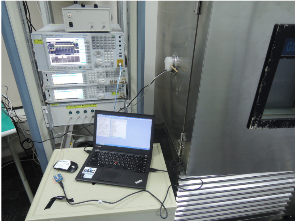
Photograph 4: Set-up for Conducted testing
