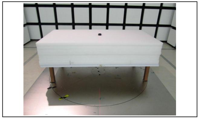
**Radiated Emission Below 1GHz Test**
