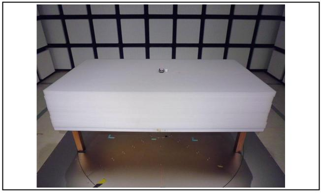
Radiated Emission Below 1GHz Test
