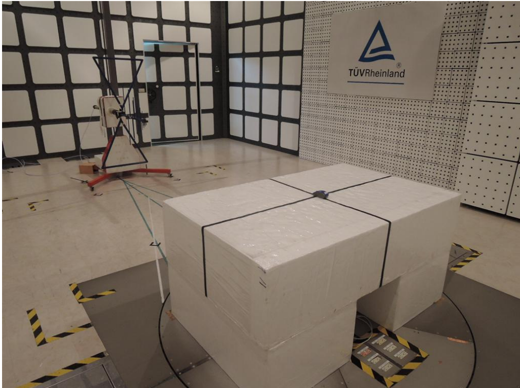
Photograph 2: Set-up for Spurious Emissions (Back View1 TX)
