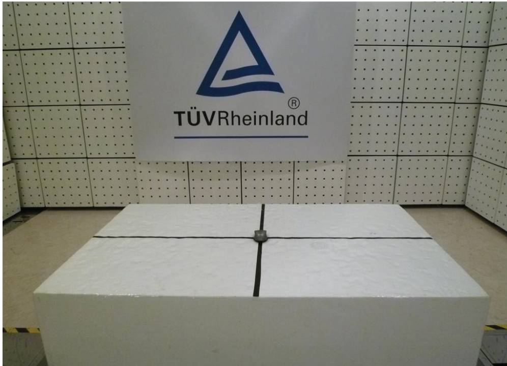
Photograph 1: Set-up for Spurious Emissions (Front View)
