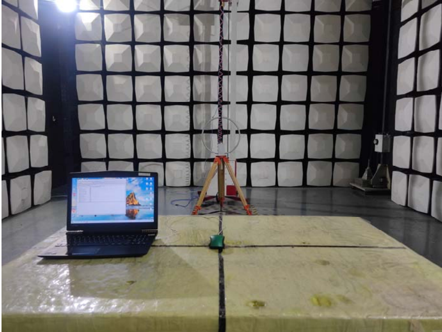
Test Photo Radiated emission (Below 30MHz)
