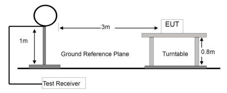
For Radiated Emission 30-1000MHz
