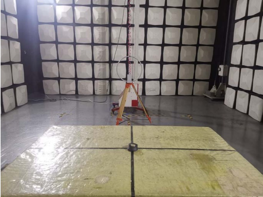
Test Photo Radiated emission (Below 30MHz)
