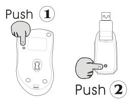
**Caution:** If you had completed the connection successfully, The LED on the receiver will be flash several times. If the ID Setting is not properly, please re set your ID again by following the above steps. Please re-setup the Rf channel since you replace batteries
