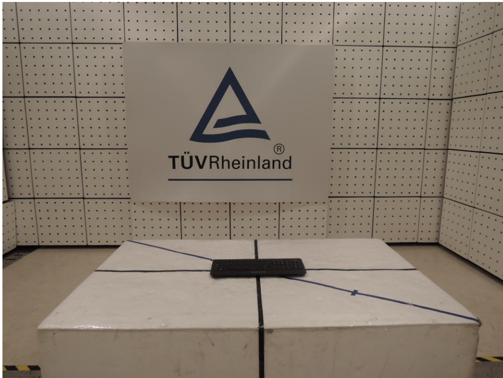
Photograph 1: Set-up for Spurious Emissions (Front View)
