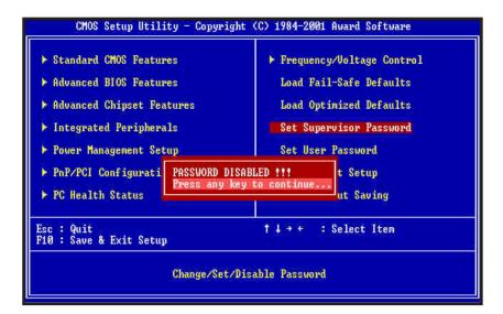
To disable password, just press <Enter> when you are prompted to enter password. A Message <<PASSWORD DISABLED!!!>> will appear to confirm the password being disabled. Once the password is disabled, the system will boot and you can enter setup freely.
