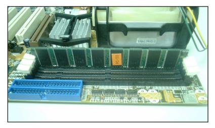
After you have set the DIMM firmly into its socket, snap the white chip holders up to lock the DIMM in place.
