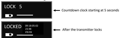
This page enables a key lock function so no parameters can be changes. When the lock page is landed on a countdown clock will begin. After 5 seconds the transmitter will lock and the display will indicated that it is LOCKED. If this screen is exited before the 5 seconds are up the transmitter will not lock.
