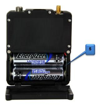
5. Battery Compartment TRXLA5 uses 2 AA batteries. Alkaline, Lithium or NiMH batteries can be used.
