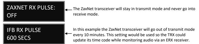
This menu sets the interval that the ZaxNet transceiver will stop sending confidence audio and search for time code.
