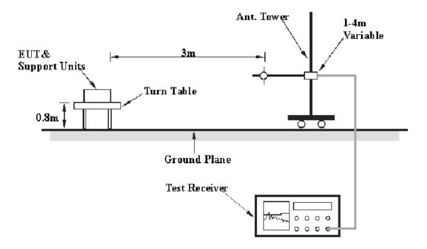
The radiated emission tests were performed in the 3 meters chamber test site, using the setup accordance with the FCC MP - 5. The specification used was the FCC part 18 limits.
