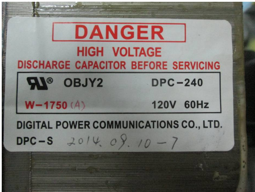
EUT – Power Transformer Label View
