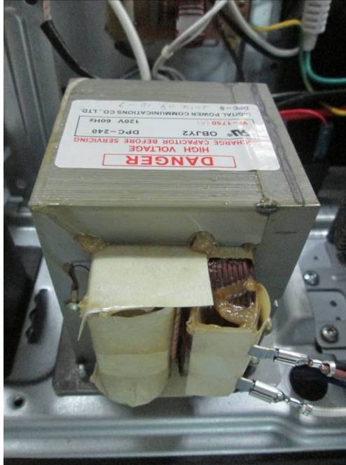
EUT – Power Transformer View
