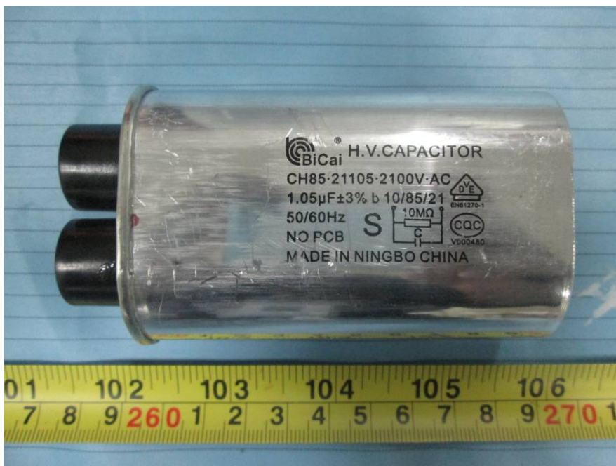
EUT – H.V. Capacitor View
