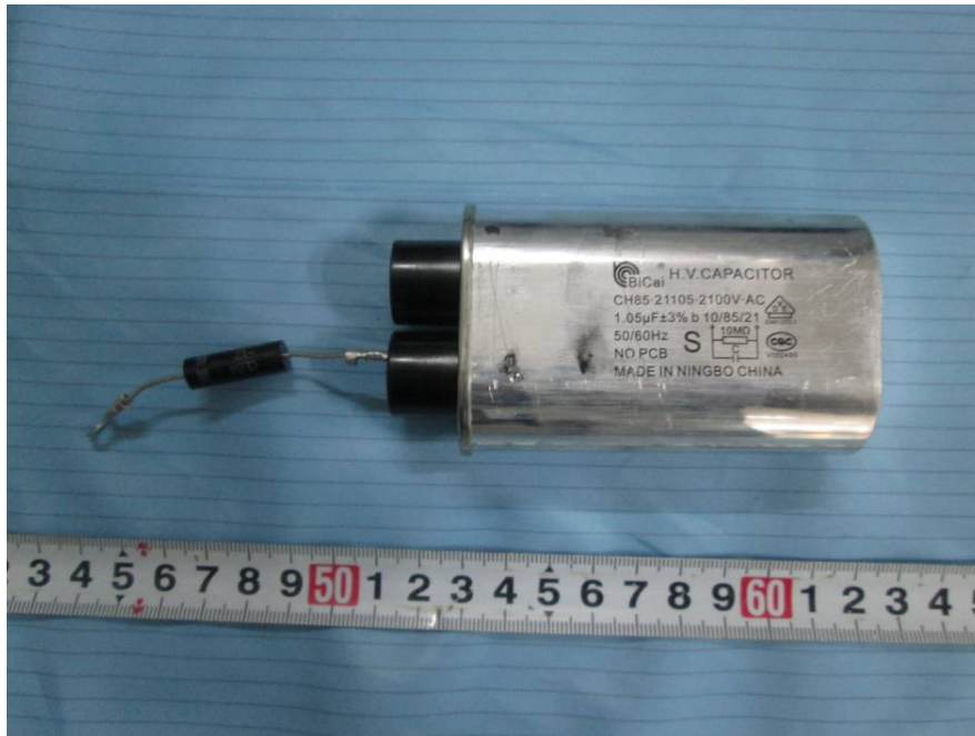
EUT – H.V. Capacitor Front View
