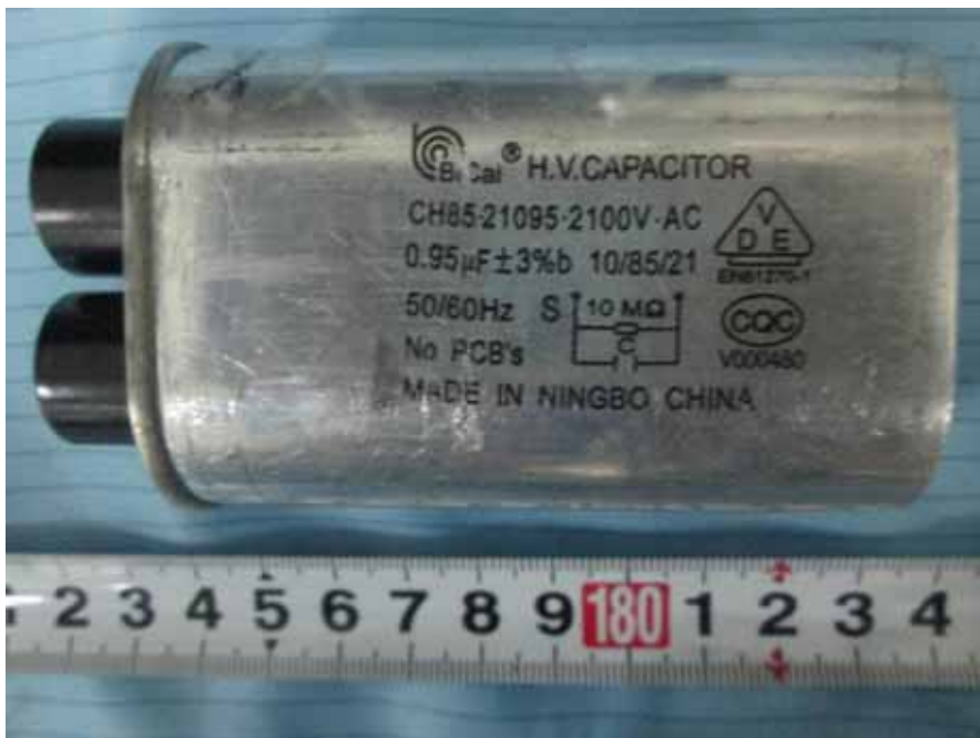
EUT – H.V. Capacitor Front View
