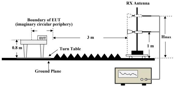
Remark: Hmax =top of EUT Spectrum Analyzer / EMI Receiver
