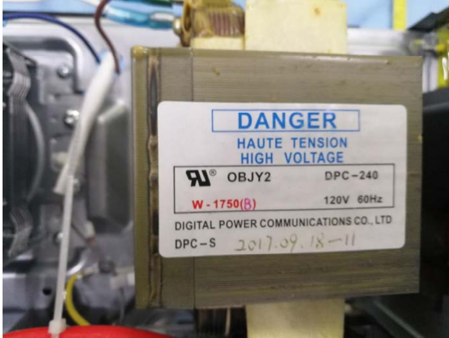
EUT – Transformer View
