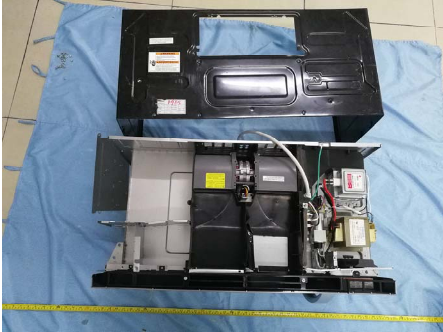
EUT – Cover off View 1
