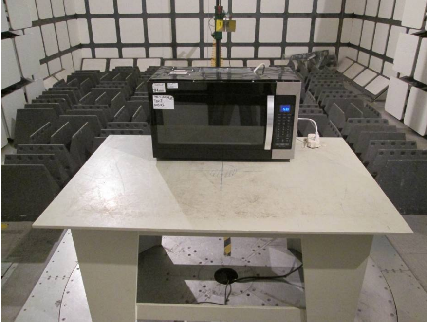
Radiated Emissions - Front View (Above 1 GHz)
