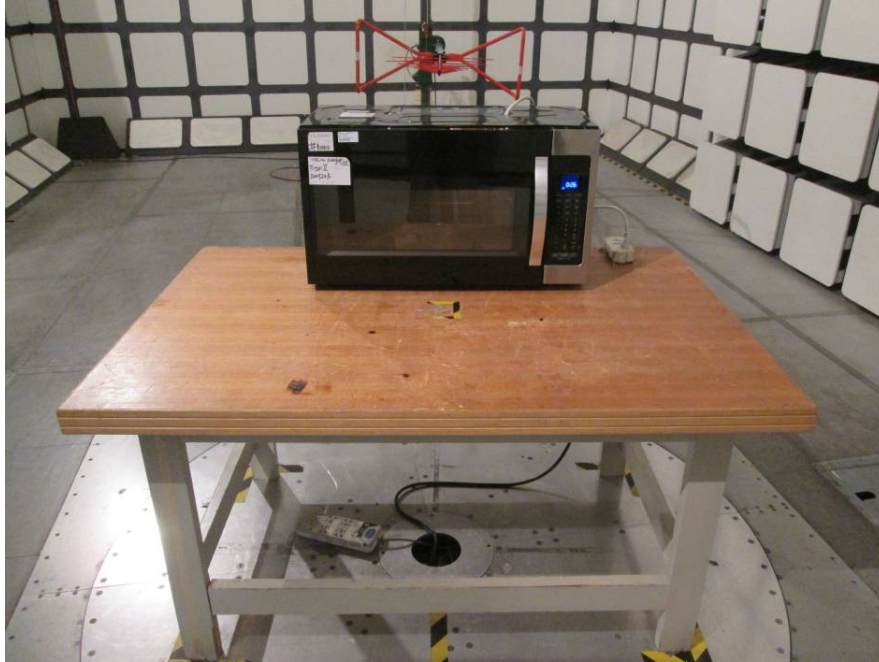
Radiated Emissions - Front View (30 MHz – 1 GHz)
