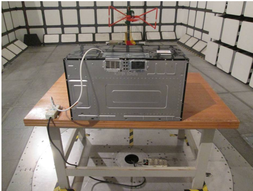
Radiated Emissions - Rear View (30 MHz – 1 GHz)
