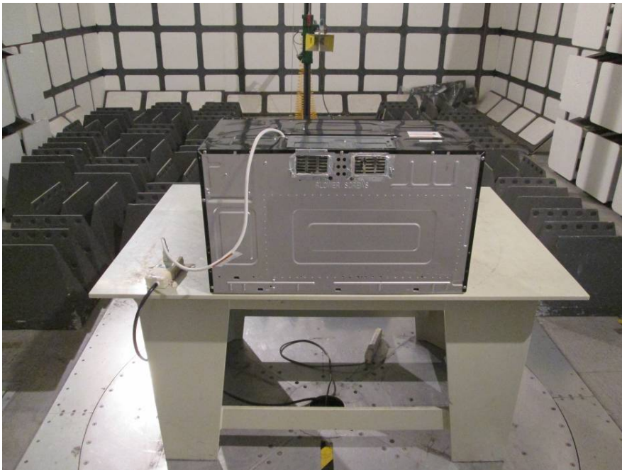
Radiated Emissions - Rear View (Above 1 GHz)
