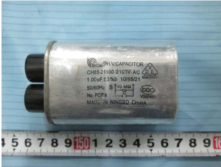
EUT – H.V. Capacitor View
