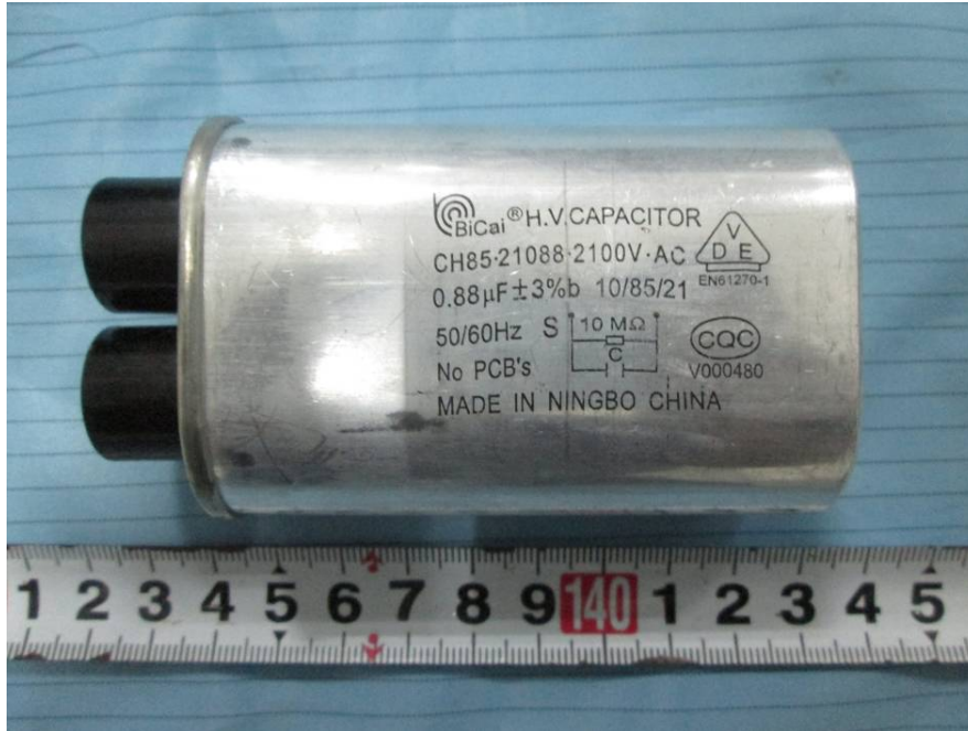
EUT – H.V. Capacitor View
