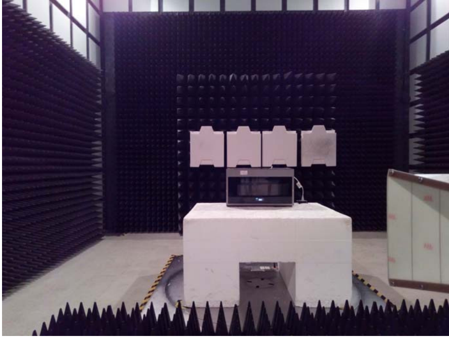
Radiated Emissions - Front View (Above 1 GHz)
