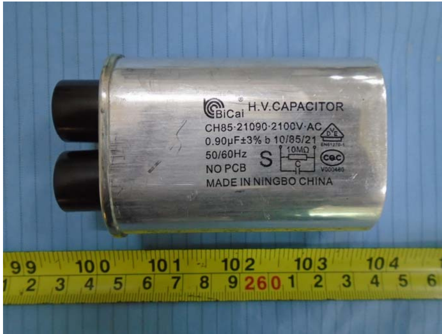
EUT -H.V. CAPACTOR View
