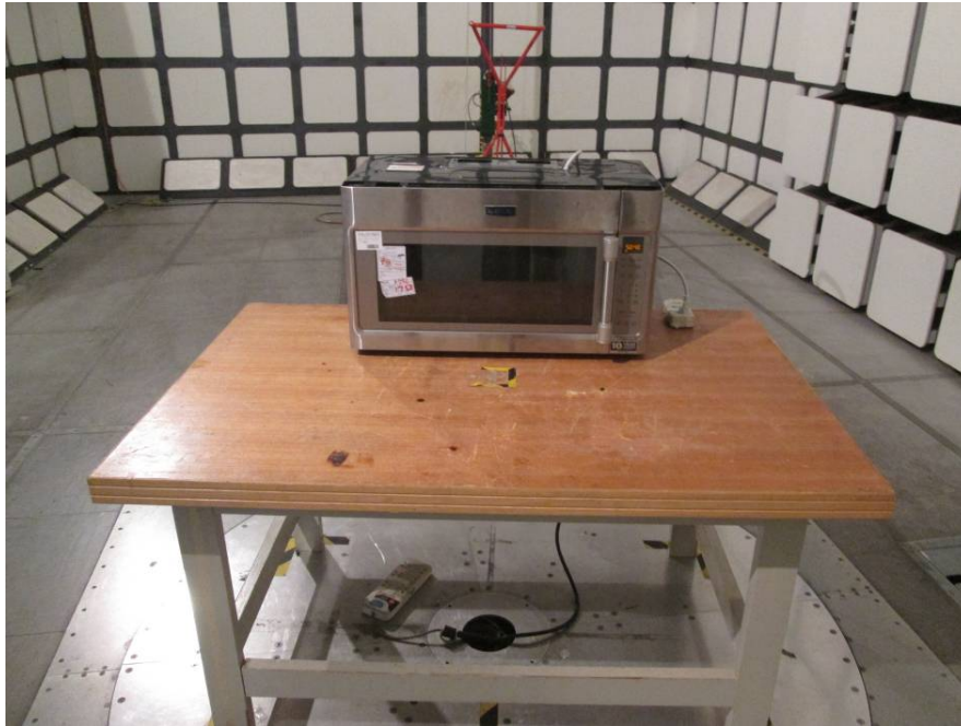
Radiated Emissions - Front View (30 MHz – 1 GHz)
