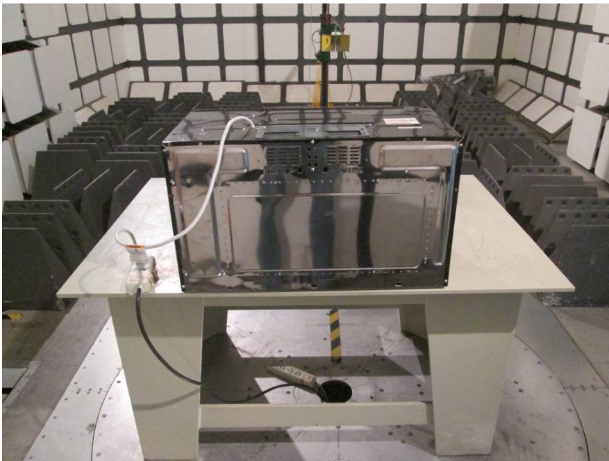
Radiated Emissions - Rear View (Above 1 GHz)
