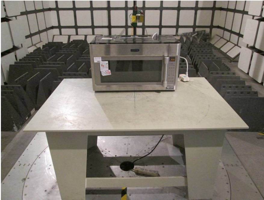
Radiated Emissions - Front View (Above 1 GHz)
