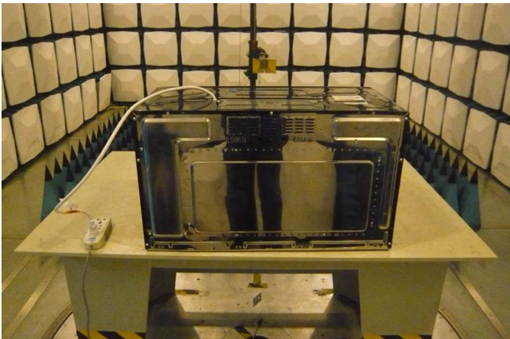
Radiated Emissions - Rear View (Above 1 GHz)
