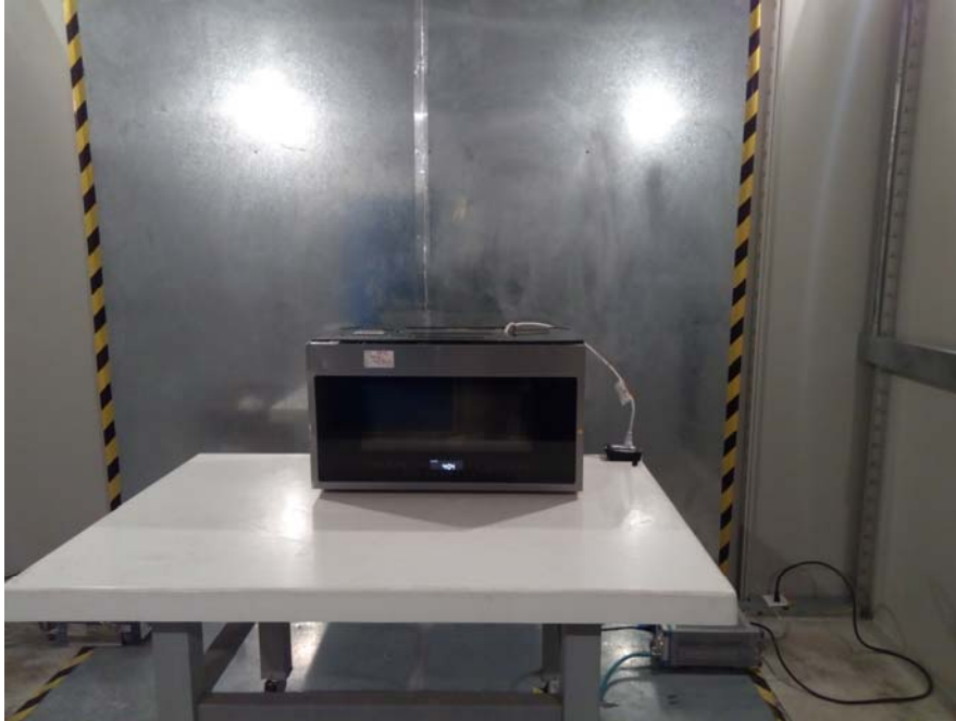
Conducted Emissions - Front View
