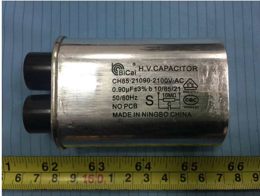
EUT -H.V. CAVAPTOR View
