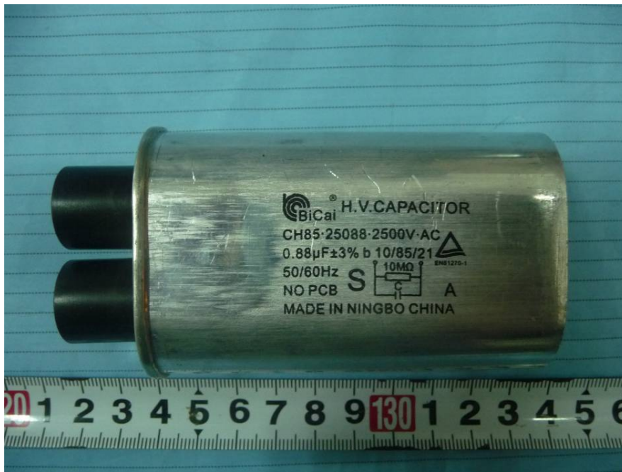
EUT – H.V. Capacitor View
