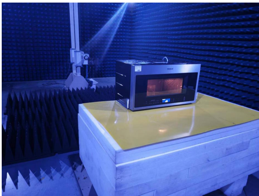
Photo of Radiated Emission Measurement Above 1GHz
