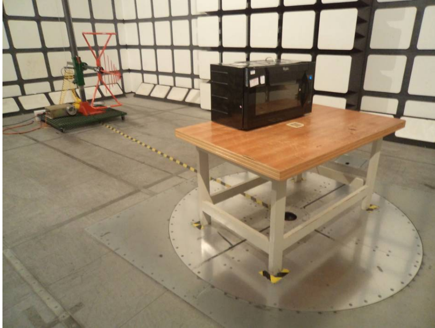
Radiated Emissions - Front View (30 MHz – 1 GHz)
