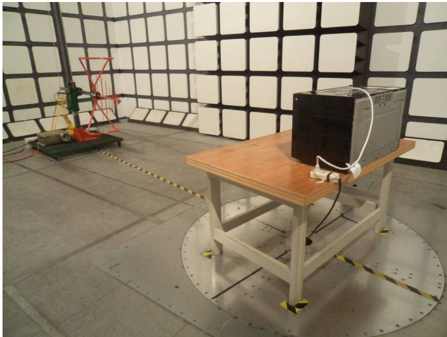
Radiated Emissions - Rear View (30 MHz – 1 GHz)
