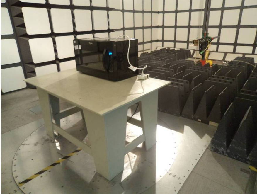
Radiated Emissions - Front View (Above 1 GHz)
