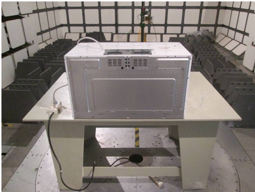
Radiated Emissions - Rear View (Above 1 GHz)
