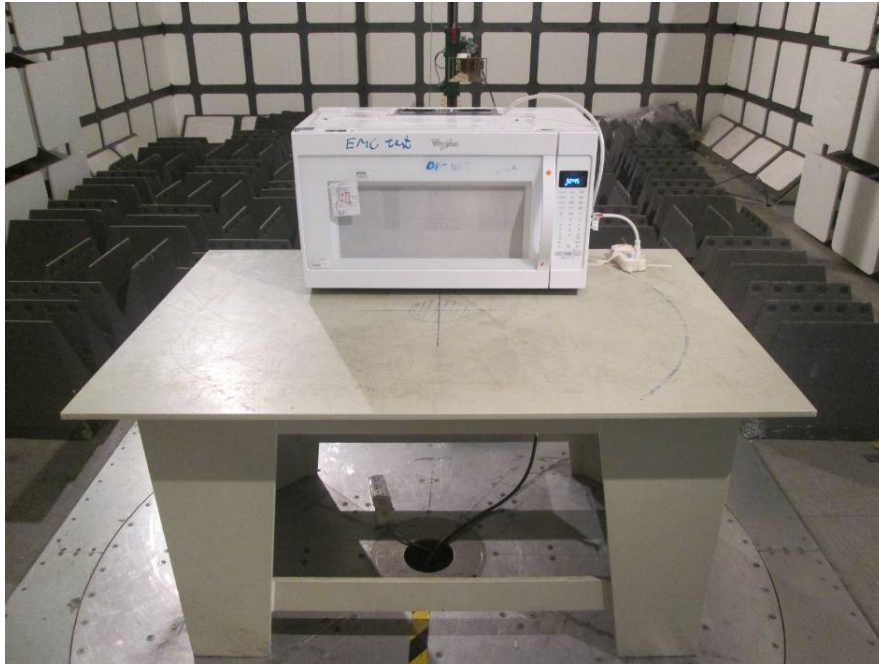
Radiated Emissions - Front View (Above 1 GHz)
