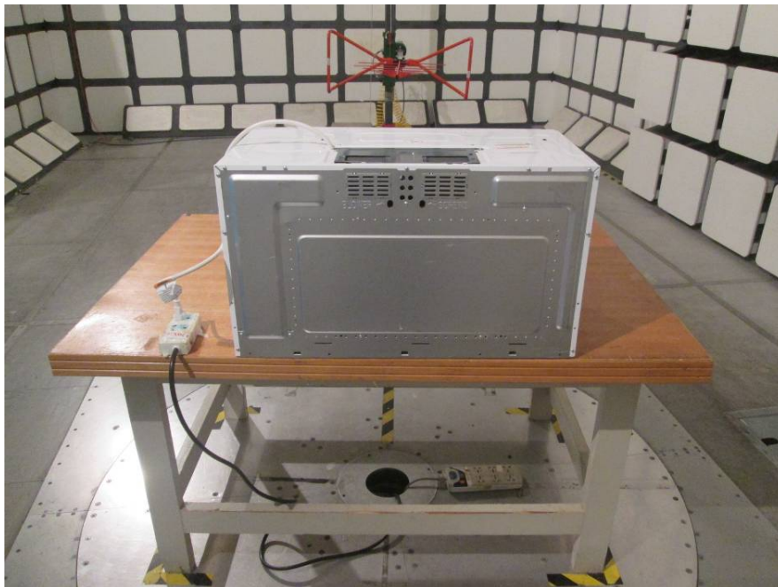
Radiated Emissions - Rear View (30 MHz – 1 GHz)
