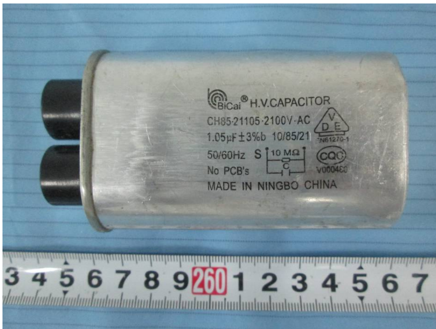
EUT – H.V. Capacitor View
