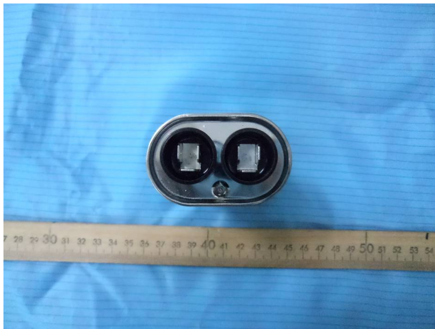
EUT – H.V. Capacitor Side View
