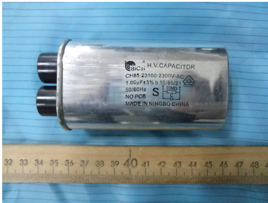
EUT – H.V. Capacitor Front View
