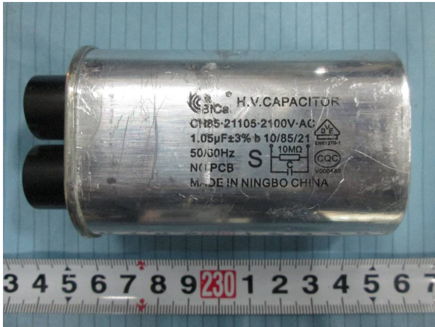
EUT – H.V. Capacitor View
