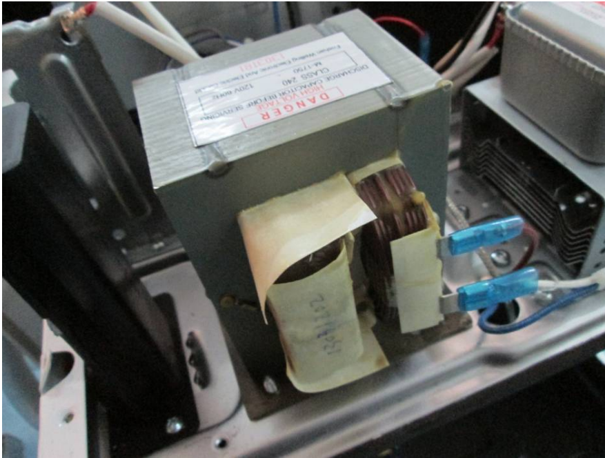
EUT – Power Transformer View
