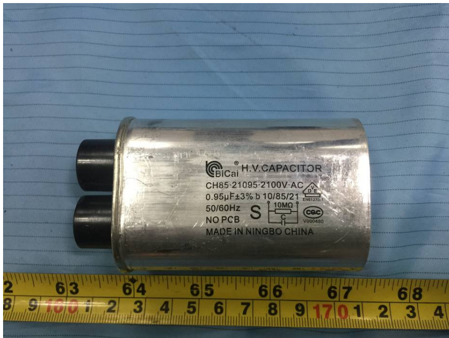
EUT –H.V. CAPACTOR View
