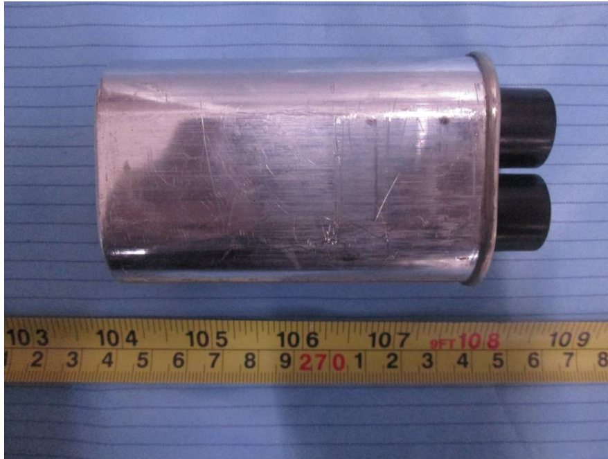
EUT – H.V. Capacitor Rear View
