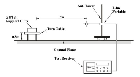
The radiated emission tests were performed in the 3 meters chamber test site, using the setup accordance with the FCC MP - 5. The specification used was the FCC part 18 limits.
