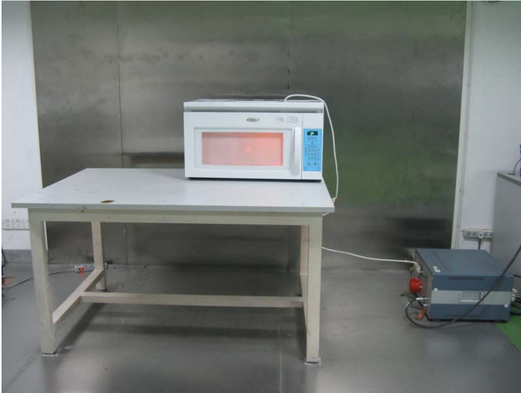
Conducted Emissions-Rear View
